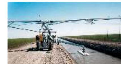
Center-feed or end-feed ditch tractor (with buried wire or above ground cable guidance)
