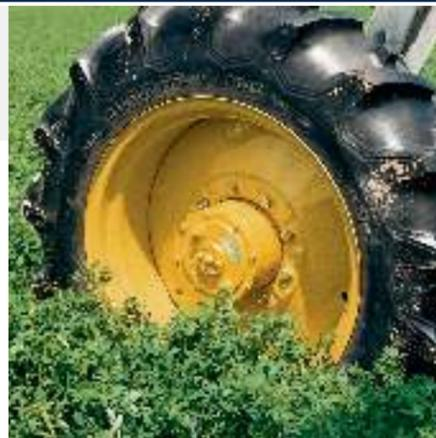
Planetary Gear Hub
