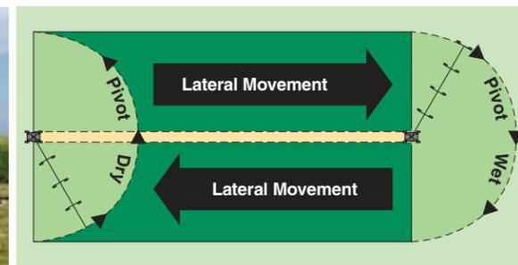
T-L's "ULTRA Linear Tractor" allows you to irrigate adjacent parallel fields with one system. The spans pivot around a stationary 4-wheel tractor using a furrow, cable, concrete ditch or buried wire for guidance. The tractor can rotate allowing the system to operate in a variety of orientations.
